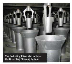
collar on the drawn edge of the tube sheet hole is also increased, firmly securing the bag's cloth.
